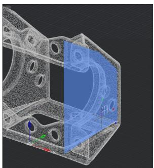
The direction of the UCS axes depends on the edge that the cursor crossed when moving to the face.
