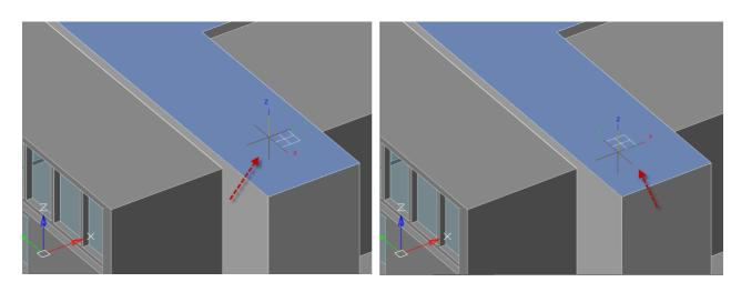
At the first mouse click, the UCS is fixed and the first vertex of the created object is set. Then you can continue to draw in the selected plane. Upon exiting the object creation command, the UCS is reset to its original orientation.
