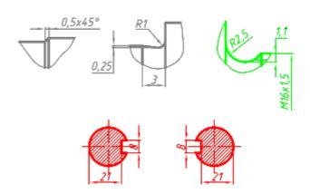
The feature creates a new dwg file that displays similar and different objects of the compared files, coloring them in several colors. In addition, you can switch off the displaying of unnecessary objects or set a transparency value for them.
