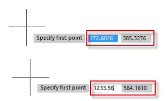
By toggling the TAB key, switch to necessary value to edit it from the keyboard. Press ENTER when done.
