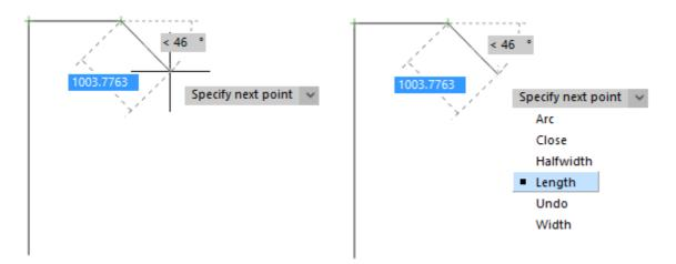
Dynamic input can be disabled by using a button DYN in the status bar or by pressing F12.
