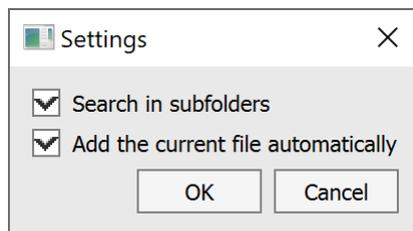
By default, the setting is enabled and when you run the **Batch File Processing (BATCHPROCESS)** command, the current drawing is added to the **Selected files** list automatically.
