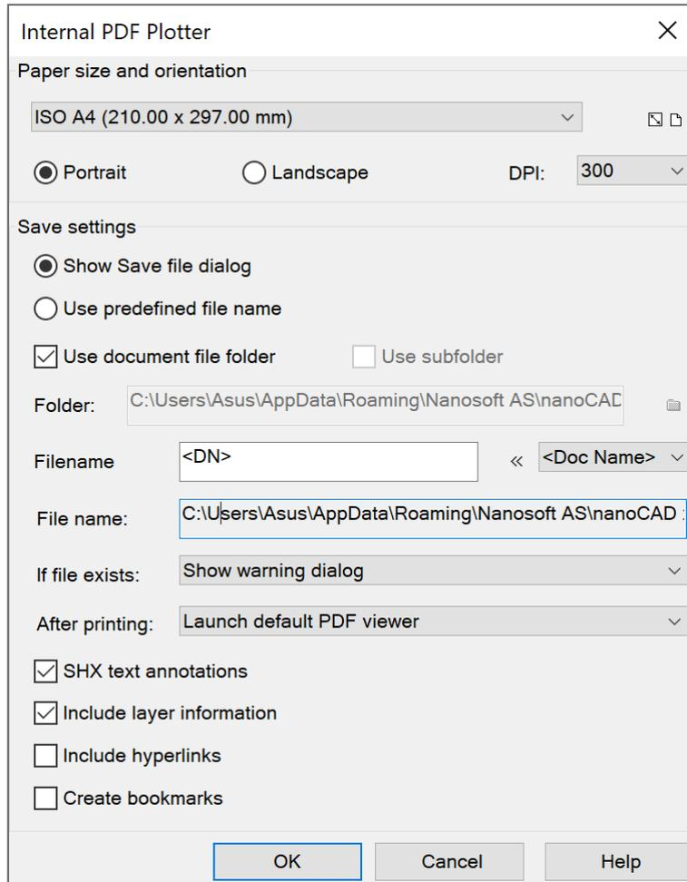
The **Include hyperlinks** option has been added to the settings dialogs for **Internal DWFX Plotter**, **Internal DWF Plotter**, **Internal PDF Plotter**, **Print as PDF**. This option converts document hyperlinks into hyperlinks in a PDF file.
