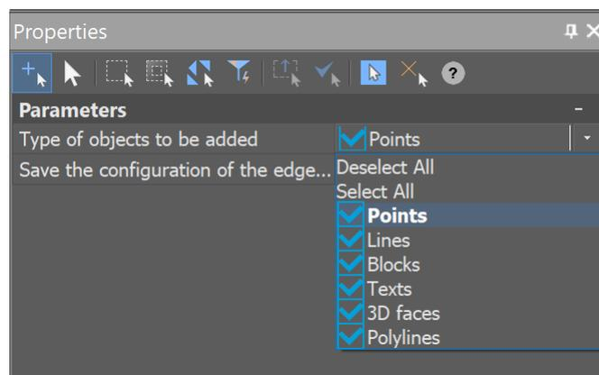
It is possible to save or rebuild triangle edges.
