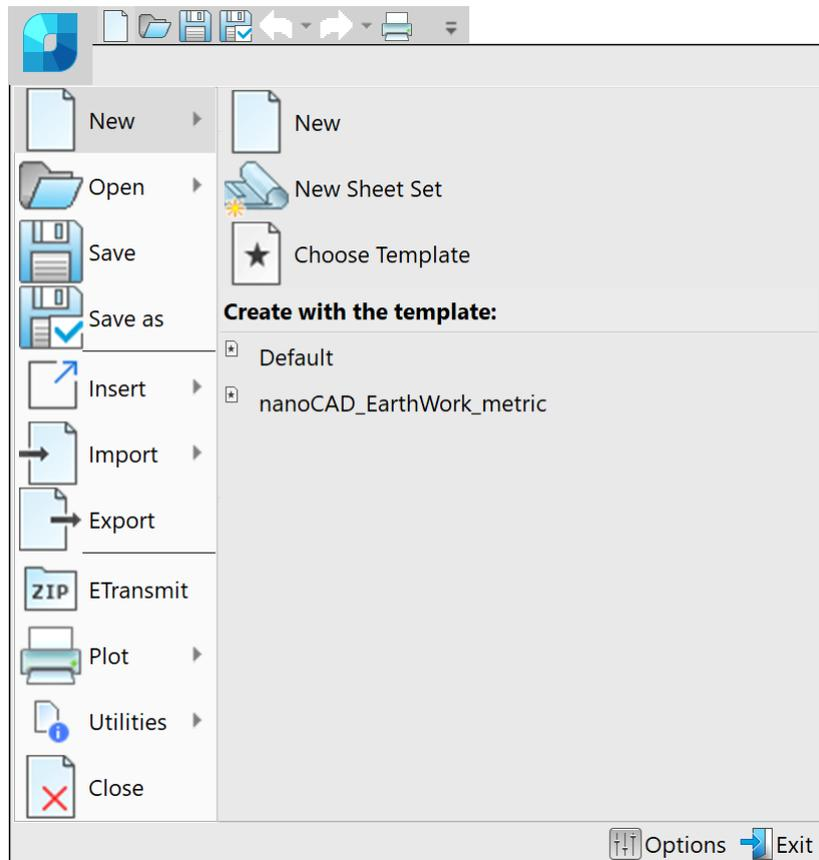
The list of templates offered for selection in the menu is limited. To select another template not presented in the list, open the **Choose template** dialog or configure the **Template Names List** in the **Template Usage** section of the **Options (OPTIONS)** dialog.
